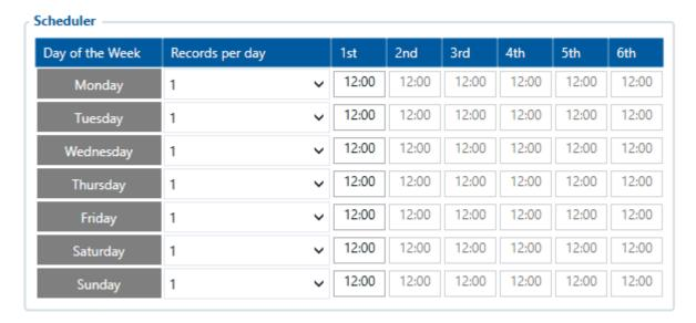
This mode is used to set up the actual schedule of data sending. Every day of the week data could be sent up to 6 times.
