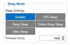
When in GPS sleep mode, TFT100 turns the GPS module off and continues making new periodic records. As a result power usage decreases, in turn saving vehicle battery.
