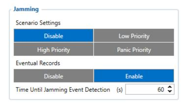
When jamming is detected the scenario is activated, an event record is generated status is changed to 1 when configured once Jamming timeout runs out. If jamming ends during timeout countdown no event will be generated. Eventual Records parameter can be configured: when it is disabled scenario status value will appear in each AVL record, otherwise it will be appended only to eventual records.
