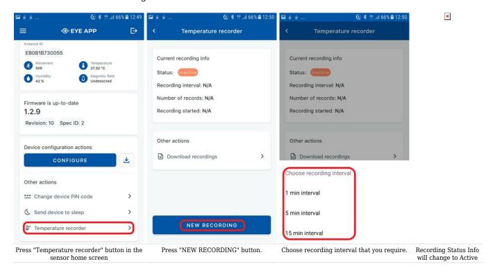
That's it! Now EYE Sensor EN12830 will be recording temperature logs to its internal memory.
