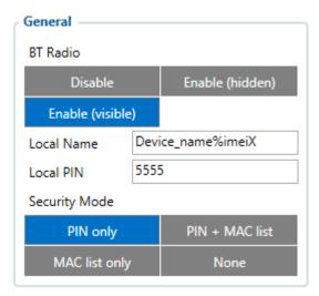
General functionality configures Bluetooth to work in slave mode. This mode allows any external device to connect to X.
