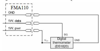
TTJ sensor pinout
