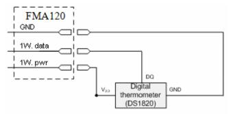
TTJ sensor pinout
