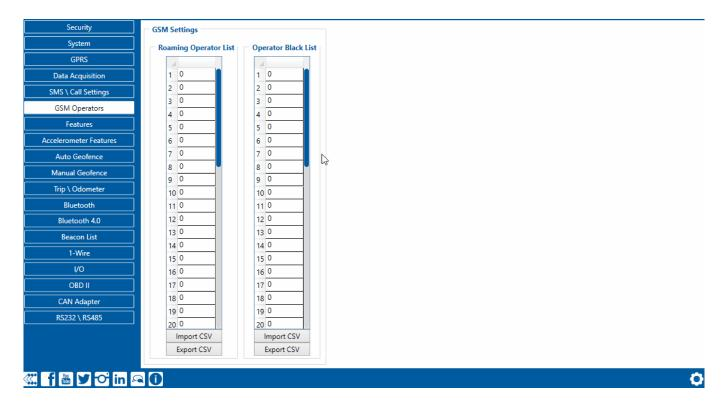
If roaming operator list is left empty, FMB1YX will automatically detect home operator. If home operator is written to the roaming operator list, it will still be detected as home operator. Any operator not in the roaming operator list (except the home operator) will be recognized as unknown operator and FMB1YX will work in Unknown mode (make sure it is configured to allow data sending – GPRS context is enabled).
