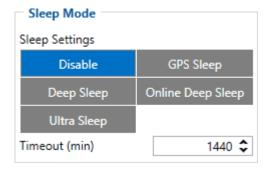
When in GPS sleep mode, FMM6YX turns the GPS module off and continues making new periodic records. As a result power usage decreases, in turn saving vehicle battery.
