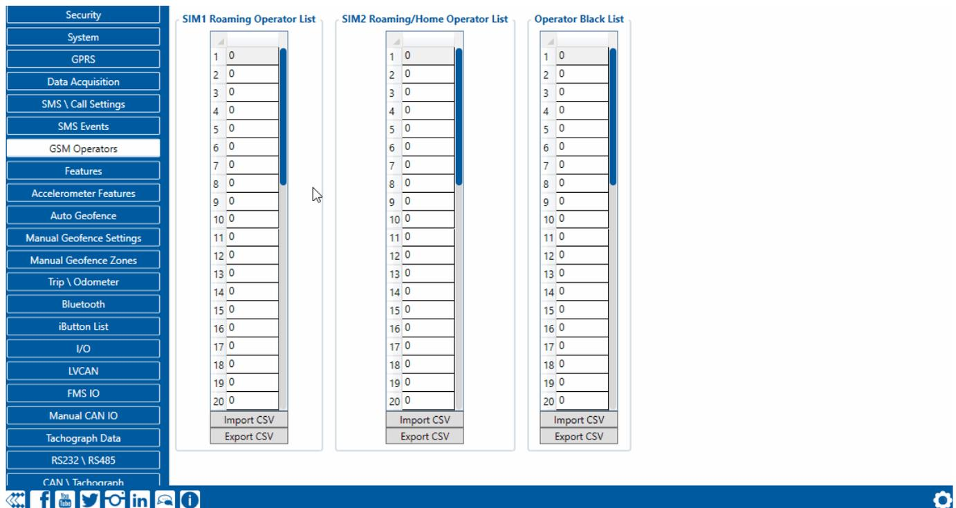
If roaming operator list is left empty, FMB640 will automatically detect home operator. If home operator is written to the roaming operator list, it will still be detected as home operator. Any operator not in the roaming operator list (except the home operator) will be recognized as unknown operator and FMB640 will work in Unknown mode (make sure it is configured to allow data sending - GPRS context is enabled).
