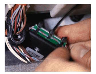
4. Connect CAN adapter **positive** and **ground** wires to the vehicle power supply lines or near FMB1YX power wires.
