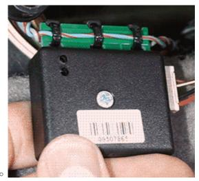
Automatic calibration process takes up to 10 seconds depending on the vehicle model. Device is calibrated properly then the LED is blinking **every 2 seconds**.
