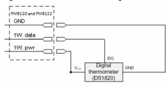
TTJ sensor pinout
