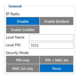
General functionality configures Bluetooth to work in slave mode. This mode allows any external device to connect to FMM1YX.
