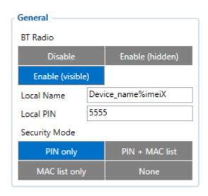
General functionality configures Bluetooth to work in slave mode. This mode allows any external device to connect to FMU1YX.
