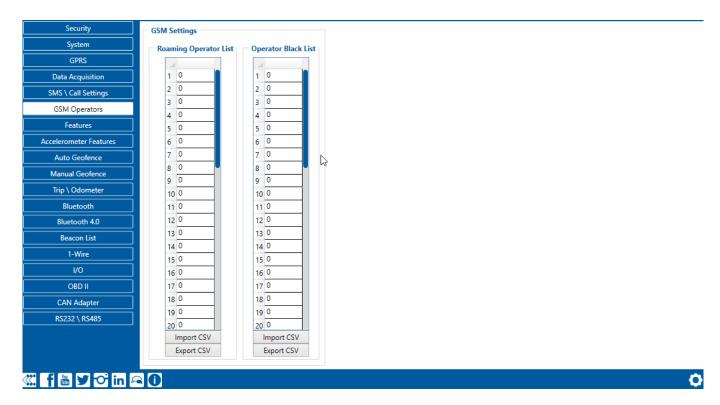
If roaming operator list is left empty, FMU1YX will automatically detect home operator. If home operator is written to the roaming operator list, it will still be detected as home operator. Any operator not in the roaming operator list (except the home operator) will be recognized as unknown operator and FMU1YX will work in Unknown mode (make sure it is configured to allow data sending – GPRS context is enabled).
