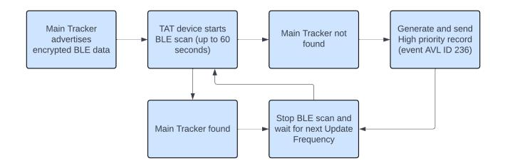
If TAT does not pick up advertised data packets from main tracker, **TAT100** generates and sends a record with AVL **ID 236** (Value 1). After sending this record, device will wait for NOTE: the next **Update Frequency** and will keep generating records with event ID 236 until main tracker is found again. No record is generated if main tracker can be located during a BLE scan.
