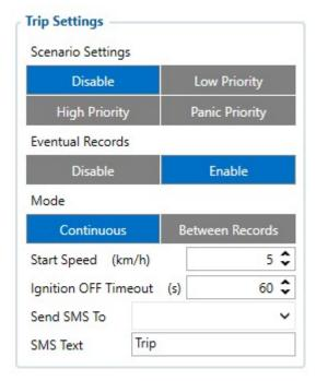
*Trip* section offers user to configure the *Trip* feature. *Trip* starts when Ignition according to *Ignition* source is ON and also 'Start Speed' is exceeded.
