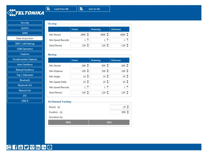
There are three available options for the activation source of tracking on demand - DIN/AIN or both. Note that, these inputs will work as buttons, rather than switches and are used to trigger the functionality, the duration of tracking on demand will not be extended if the activation source status is high for a period of time.
