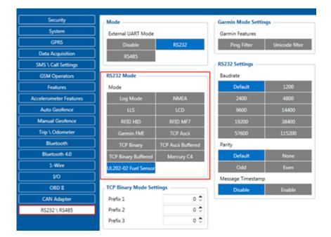
To receive UL202 Fuel Sensor information to the configured server, the Ultrasonic UL202-2 Fuel level and status have to be enabled in the "I/O" section.
