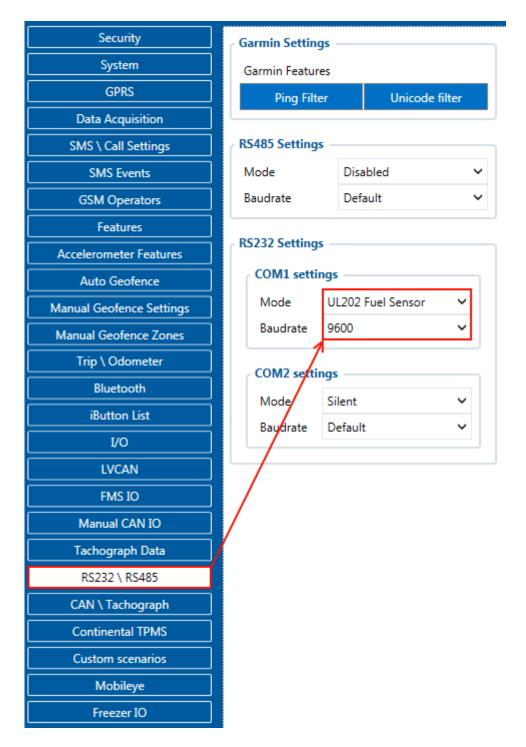
To receive UL202 Fuel Sensor information to the configured server, the Ultrasonic UL202 Fuel level and status have to be enabled in the "I/O" section.
