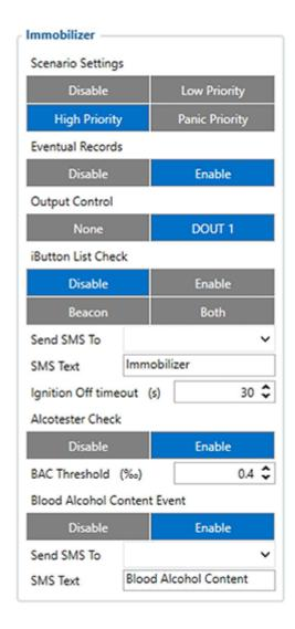
GPS tracker RS-232 mode with breathalyser Mercury model has to be configured allowing corresponding data communication between two devices. To provide an electrical connection, USB connector pins TXD and GND of Alcovisor Mercury should be connected to RS-232 port pins RXD and GND of FMC125 tracker accordingly. Also, the breathalyser unit has to be calibrated as advised by its manual.
