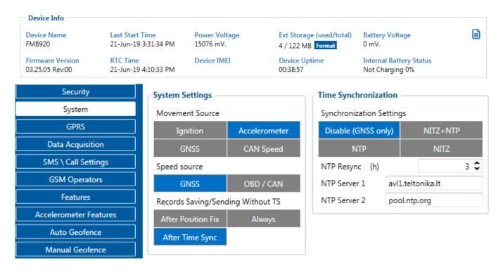
7.2. If you have configured your device to send records after the position fix, and you are testing your device on the table indoors, the device may not be able to get a GPS fix and therefore will not save or send any records to the server.
