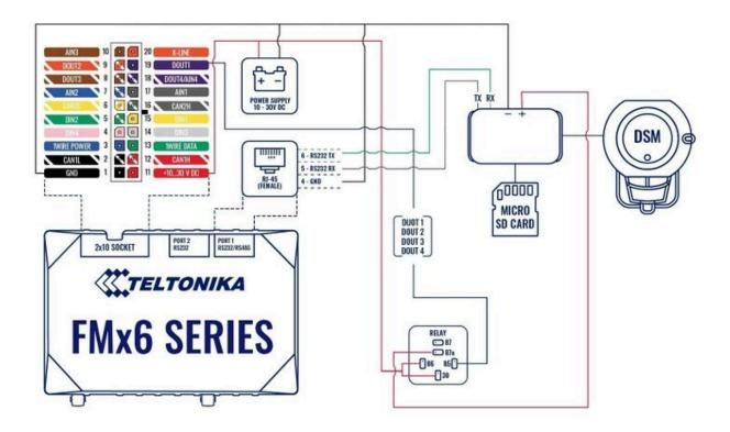
**Two cameras FMC650 Installation with Ignition Source**. To connect the two cameras to the FMC650 device, you have to make sure to connect 4 PIN's of the camera to the PIN's of your device correctly.
