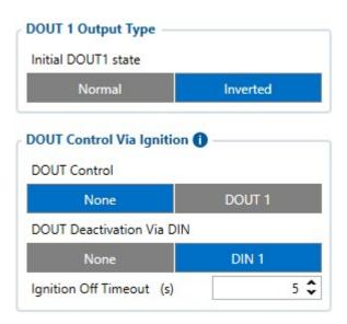
DOUT 1 Output Type has selections of either normal or inverted. Selecting inverted will make the DashCam turn on when the DOUT1 state will be 0 and turn off the the state changes to 1 and vice versa. This is recommended as inverted selection will turn on the camera upon turning on you FMx
