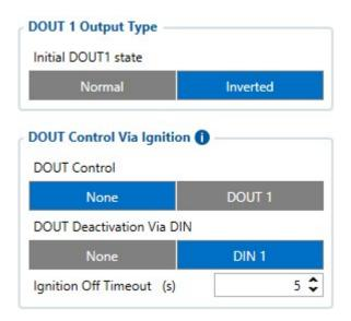
DOUT 1 Output Type has selections of either normal or inverted. Selecting inverted will make the dualcam turn on when the DOUT1 state will be 0 and turn off the the state changes to 1 and vice versa. This is recommended as inverted selection will turn on the camera upon turning on you FMx device. When 'Normal' is selected, you will need to send an SMS message to the device requesting to turn on DOUT1 every time **IF DOUT control via ignition** is not turned on.
