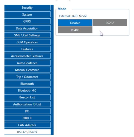
• **Do not forget** to configure *DualCam* server information. In **RS232\RS485** fill in **DualCam Server Settings** with *Domain* and *Port* entries.
