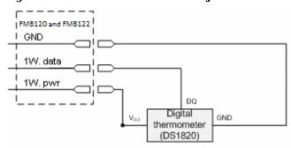
TTJ sensor pinout
