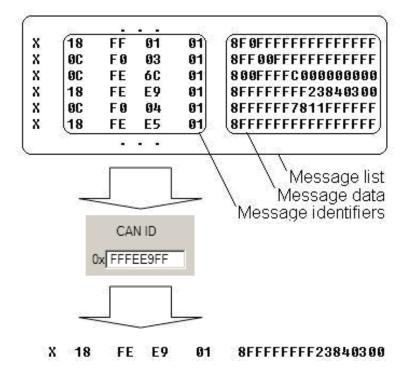
When certain message is filtered, FM6320 checks which data bytes should be sent to server. Document indicates that 5-8 bytes are used in FMS standard.
