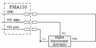
TTJ sensor pinout
