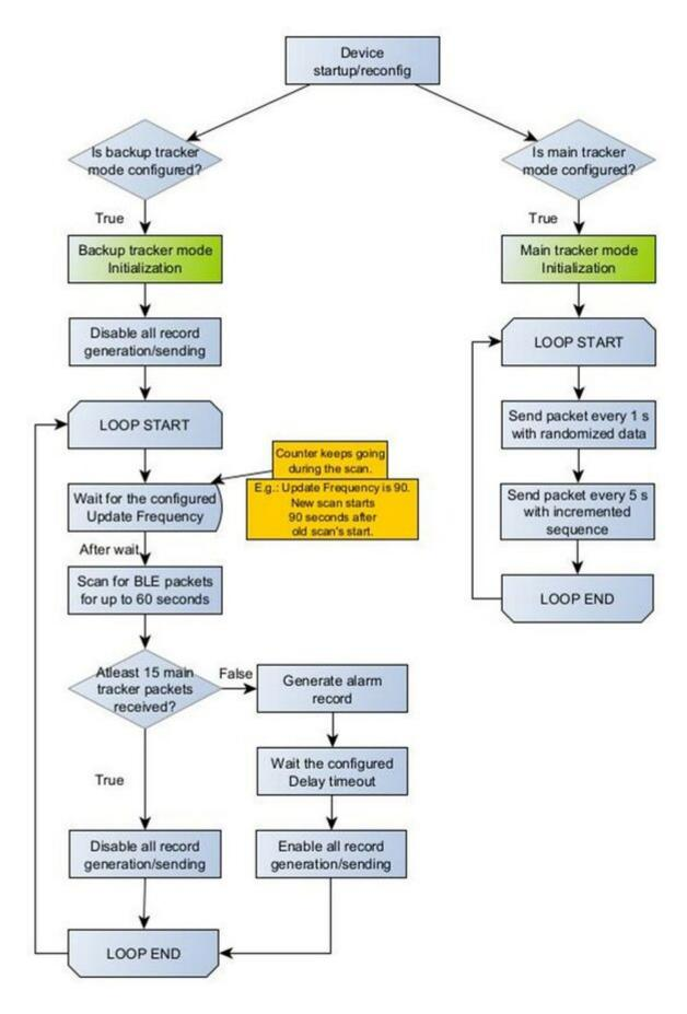
Each time the device is starts up or gets reconfigured, it checks if either main or backup tracker modes are enabled on the current configuration.
