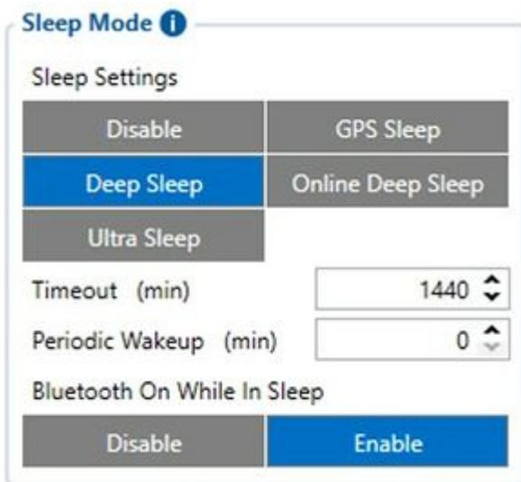
Note: In case when during scan after wakeup no BLE devices will be found FMB will be active for configured scan duration time in Bluetooth 4.0 tab. After that timeout FMB will go to sleep state.
