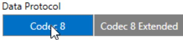
In *Data Protocol* settings user can choose which protocol version ([Codec 8](#) or [Codec 8 Extended](#)) will use for data sending to the server.
