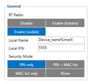
General functionality configures Bluetooth® to work in slave mode. This mode allows any external device to connect to FMB003.
