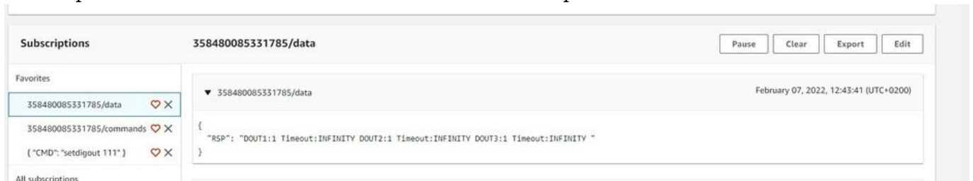
Figure 32. Response to a command in the data topic, the command was published in command topic
