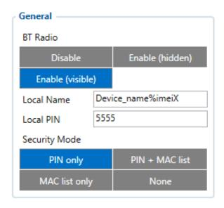
General functionality configures Bluetooth® to work in slave mode. This mode allows any external device to connect to FMB020.
