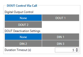
The scenario is activated and digital output is ON when a call is received from a number that is on the authorized numbers list.
