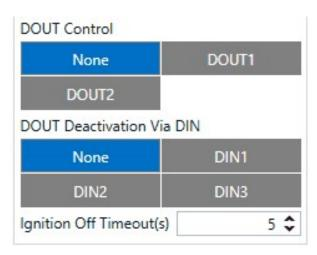
This feature allows direct control of DOUT by configured ignition source status. When enabled, the function will start to monitor ignition status, and once the ignition changes state from On to Off after configured Ignition Off a timeout, selected DOUT (Digital Output) will be turned On.
