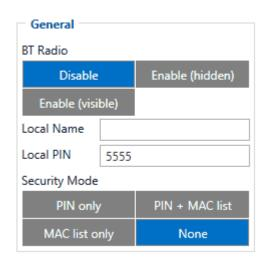
General functionality configures Bluetooth @ to work in slave mode. This mode allows any external device to connect to FMB150.
