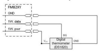
TTJ sensor pinout
