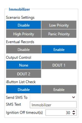
If *DOUT Control* is disabled, the scenario will only generate events without digital output activation. If *DOUT Control* is enabled DOUT1/DOUT2 turns ON if ignition turns ON (*Ignition Source* is configured to 1). After any iButton ID (or RFID card) is attached, DOUT1/DOUT2 turns OFF. After iButton identification configured *Ignition Source* can be turned OFF (*Ignition Source* is configured to 0) for no longer than 30 seconds, otherwise, the immobilizer must be repeated. If the *iButton List*
