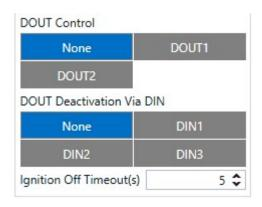
This feature allows direct control of DOUT by configured ignition source status. When enabled, the function will start to monitor ignition status, and once the ignition changes state from On to Off after configured Ignition Off a timeout, selected DOUT (Digital Output) will be turned On.
