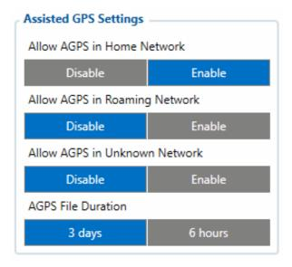
Assisted GPS is a feature that significantly improves the time to first fix. It works by providing the necessary data to the device via the cellular network instead of the slow satellite link, essentially "warming up" the receiver for a fix.
