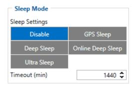
When in GPS sleep mode, FMB208 turns the GPS module off and continues making new periodic records. As a result power usage decreases, in turn saving vehicle battery.
