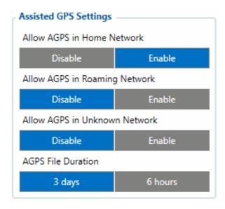
Assisted GPS is a feature that significantly improves the time to first fix. It works by providing the necessary data to the device via the cellular network instead of the slow satellite link, essentially "warming up" the receiver for a fix.
