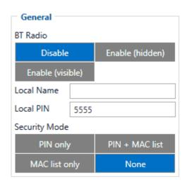
General functionality configures Bluetooth @ to work in slave mode. This mode allows any external device to connect to FMB209.
