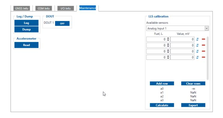
• Dump - after button is pressed, the device starts to download .dmp logs and configuration .cfg from device in compressed archive.
