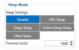
When in GPS sleep mode, FMB240 turns the GPS module off and continues making new periodic records. As a result power usage decreases, in turn saving vehicle battery.
