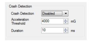
If Crash Detection is enabled, it monitors acceleration on each axis which helps to detect an accident. Threshold and Duration values are set depending on the impact magnitude that is required to be detected. FM63XY can detect events ranging between a slight tapping on the device and a severe accident.
