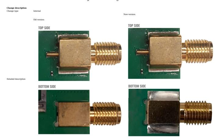
Change reasons/Description In order to increase the structural rigidity and unify the manufacturing process of Teltonika IoT Group devices, SMA connector will be soldered on the top side of PCB (same as before) and on the bottom side of PCB (performed additionally).
