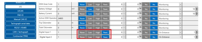
In the scenario shown in the above picture when panic record is made (generated by *Digital Input 1* or *Digital Input 2*) internal 90 seconds timer will start to tick and if in that timeout device will not send the record through GPRS network it will be sent with Iridium satellites.
