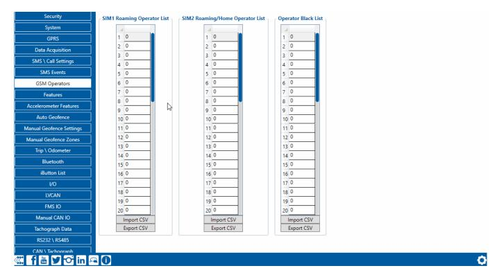
If roaming operator list is left empty, FMB641 will automatically detect home operator. If home operator is written to the roaming operator list, it will still be detected as home operator. Any operator not in the roaming operator list (except the home operator) will be recognized as unknown operator and FMB641 will work in Unknown mode (make sure it is configured to allow data sending – GPRS context is enabled).
