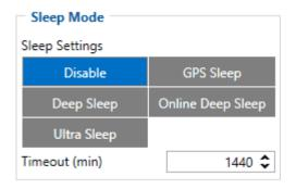
When in GPS sleep mode, FMB641 turns the GPS module off and continues making new periodic records. As a result power usage decreases, in turn saving vehicle battery.
