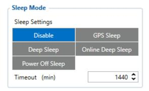
When in GPS sleep mode, FMB930 turns the GPS module off and continues making new periodic records. As a result power usage decreases, in turn saving vehicle battery.
