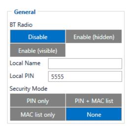
General functionality configures Bluetooth® to work in slave mode. This mode allows any external device to connect to FMB962.
